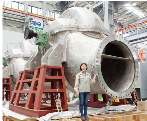
Cooling Water Pump (BB1)
